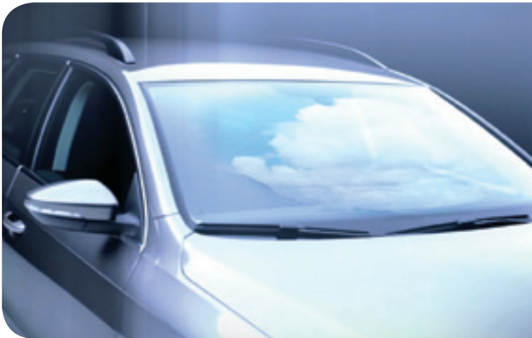
60% of the sun's heat is reflected to the outside, and the cabin stays cool as only 40% adds to the heat build-up of the car.
