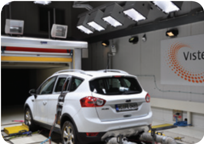
Glass properties being tested in a climate tunnel.
