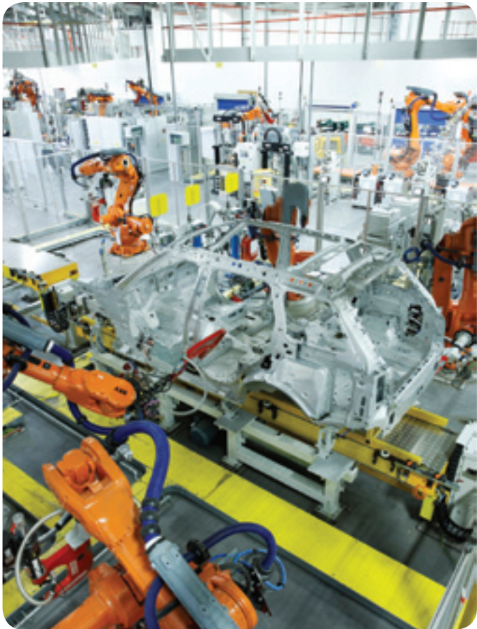
The world's largest aluminum body shell – a body-in-white on the Solihull production line.
