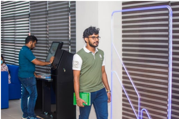
Figure 2: RFID self-check machine with the RFID security gate
